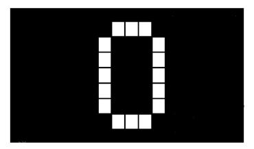
Here right char blinks. Now it can be changed by pushing INC ( $\uparrow$ ) and DEC ( $\downarrow$ ) buttons. Any number or letter can be chosen. After selecting right char, push ENT shortly and left char starts to blink. In the same way left char is set. Then select floor and signal color by pushing ENT and change with INC ( $\uparrow$ ) and DEC ( $\downarrow$ ) buttons. If no color selected to signals, then floor color displays.
