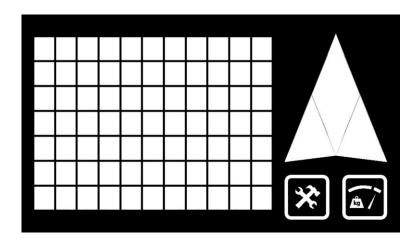
After initialization, software version number and ID (in CANBus) is displayed first. Then inputs are evaluated and related character(s) are displayed according to stored settings. If no input is connected or all connected inputs are passive then floor 0 character(s) are displayed. (In 7-Segment Mode if no input is connected or connection is wrong then no character displays; if no communication established in CANBus mode, then "CE" displays)
