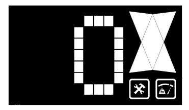
This display shows upper menu of Floor 0 (bottom floor). To edit Floor 0 display data, push ENT shortly and enter sub-menu.
